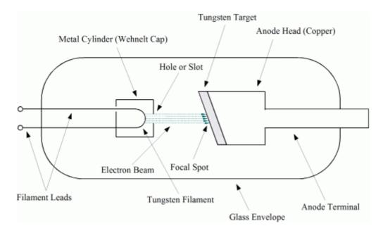
The filament is electrically heated (>2200 K) and emits electrons (thermionic emission). The electrons are focused on the target by means of a hole or slot in a metal cylinder surrounding the filament (Wehnelt cap). In contrast to a cold-cathode tube, the anode current of a Coolidge tube is virtually independent of the anode voltage and is solely controlled by the filament current.
