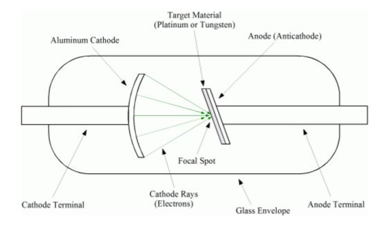
The radiation thus emitted is omnidirectional, but a significant part of it is absorbed by the target metal and the anode head. The target surface usually forms an obtuse angle (45...85°) with the tube axis. This enables a greater part of the radiation to exit the tube sideways (penetrating the glass envelope).
